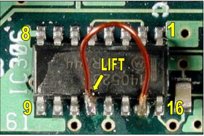
Figure 2: T1511 CCM PCB modification completed
