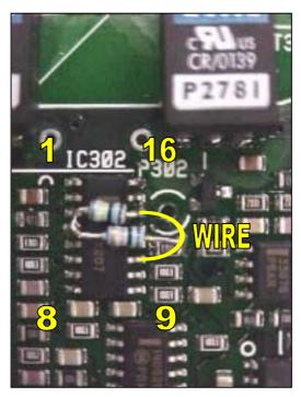
Figure 4: T1711 CMM wire modifications completed
